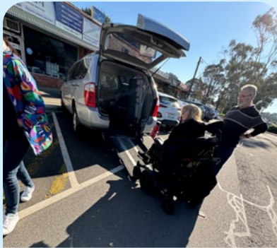
Accessible car park too short, therefore PMDs have to enter and exit the car in the roadway. FTG
