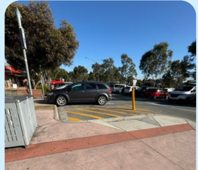
Share zone adjacent to accessible car park which is connected to the footpath and protected by a visible bollard. WM
