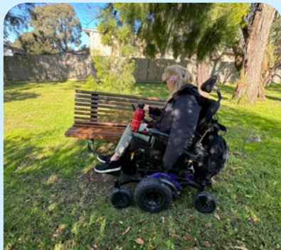
No concrete pad around bench. No handrails to assist person getting up. FTG
